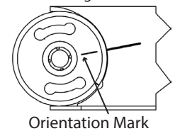
Figure 1. (Wide) Bushing Orientation Draw Reference Line on Beam Before Bushing is Removed
