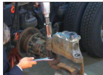
Figure 71 – Remove the Long Guide Pin
