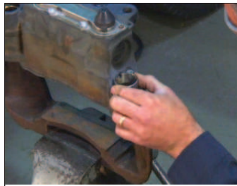
Figure 78 – Position the New Bushing
