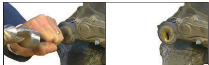
Figure 63 – Punch Guide Pin Cap (10)
