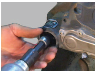
Figure 67 – Remove the Caliper Bolts
