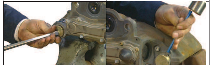
Figure 65 – Pry to Remove Guide Pin Cap (10)
