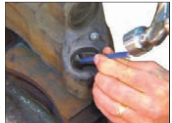
Figure 74 – Remove the Tab that Holds the Bushing in Position
