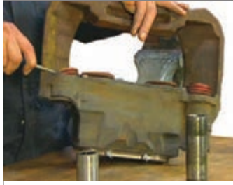
Figure 69 – Remove the Retaining Rings, Guide Pins, and Boots
