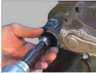
Figure 68 – Remove the Caliper Bolts
