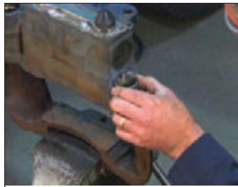
Figure 79 – Position the New Bushing
