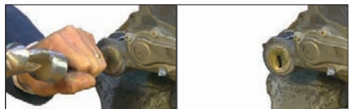
Figure 64 – Punch Guide Pin Cap (10)
