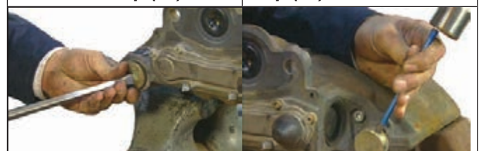
Figure 66 – Pry to Remove Guide Pin Cap (10)
