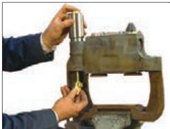
Figure 71 – Install the Removal Tool
