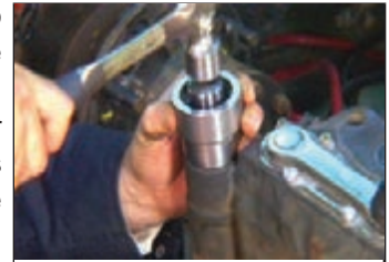
Figure 86 – Boots Must Be Compressed Fully During Cap Installation
