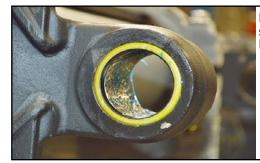
Inspect cam bearing inside the spider; cam bearing seal; and, thrust washer for damage.
