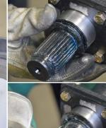
Insert splined end of cam through outboard side of cam enclosure. Secure cam in cover with flat washer and snap ring.
