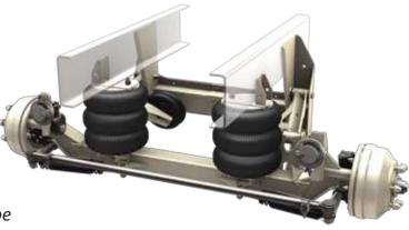
RSS-232-13K 13,200 lb. capacity 13.5" total travel, 10" up travel 30 degree wheel cut Fits ride heights 7" to 18" 842 lbs. - lightweight wheel ends 876 lbs. - standard wheel ends Compact 22.0" mounting envelope
