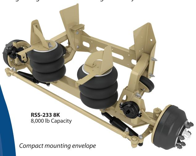
Assembled with Huck® fasteners for reduced maintenance
