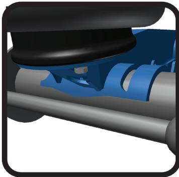
Patented contoured axle seat optimizes axle weldment by decreasing stress concentrations. No u-bolts required.
