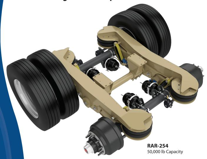
Weld-on pedestal mounts for trunnion height customization
